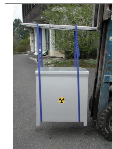
Fig. 6 Container transport on straps
